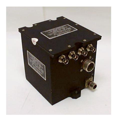
Systems & Electronics, Inc. (SEI) Signal Data Converter (SDC), CV-4318/ASH-37 offers the capability of acquiring data from dual MIL-STD-1553 busses and has a real time clock. The data acquired from these busses and real time clock are transmitted to SEI's multiplatform Structural Data Recording Set (SDRS), AN/ASH-37(v) via RS-232. The SDRS is a multi aircraft data acquisition system. The unit presented in this technical data sheet is currently on the Navy's EA-6B aircraft.
