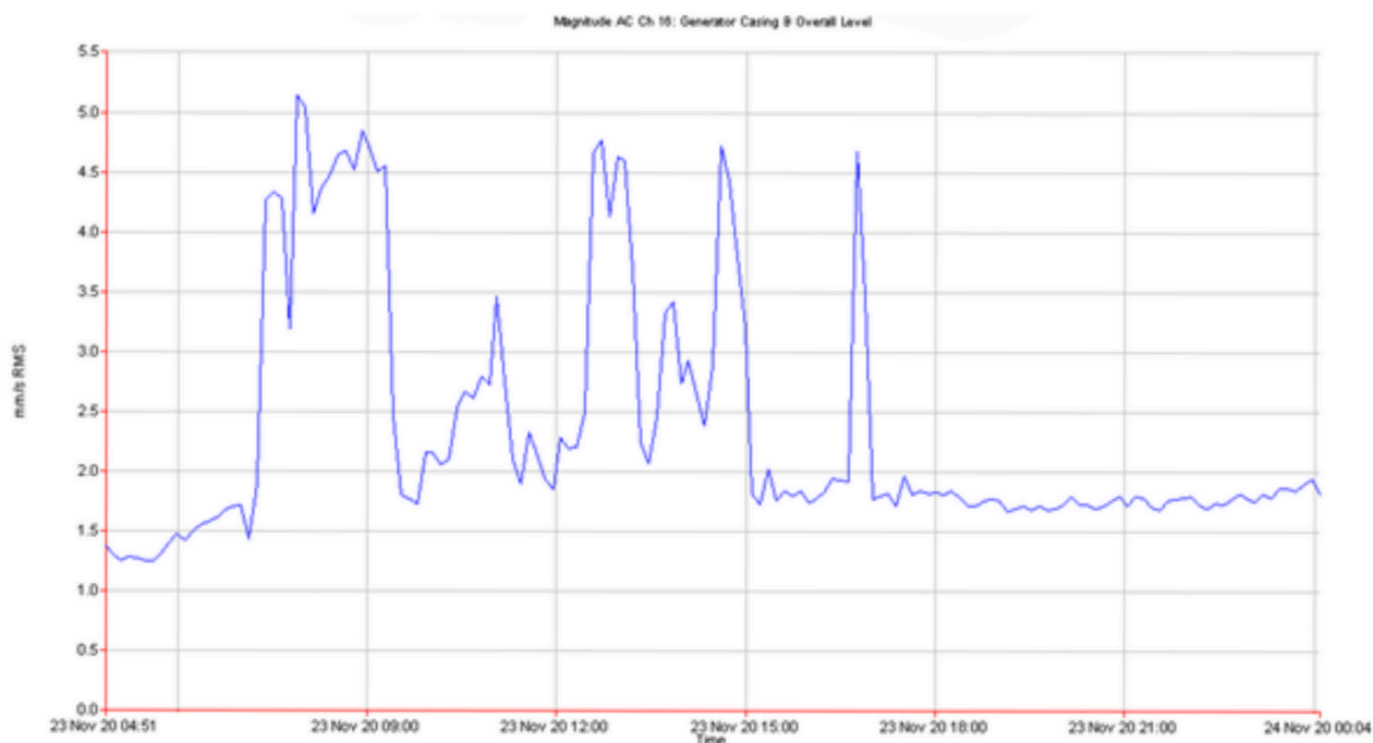
Figure 5: Shows overall vibration trend for 20 hours showing intermittent nature of issue.
