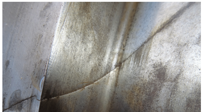
Excessive amplitudes of torsional vibrations can lead to shaft cracking without warning.
