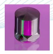
The A/800 is the highest sensitivity accelerometer in the DJB range. Using multiple shear plates and large masses the 9000pC/g sensitivity makes it perfectly suited to seismic surveys and other micro g level measurement – virtual immunity to strain input side effects provides guarantee of low frequency, measurement integrity. System noise level of 10<sup>-2</sup>pC is equivalent to 1mg. With bandwidth restricted to 1 kHz, noise floor should be significantly below this.
