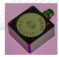
The AMB range of accelerometers are Biaxial MEMS (micro electro mechanical system) DC response voltage output devices for testing at low frequency vibration measurement from DC (0Hz) and above. They are Biaxial (measuring in 2 directions simultaneously) variable capacitance design. The AMB/20.100C has a 4 pin <sup>1</sup>/<sub>4</sub>-28UNF side entry connector.
