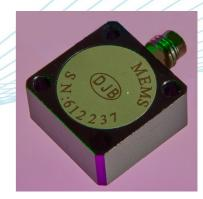
The AMB range of accelerometers are Biaxial MEMS (micro electro mechanical system) DC response voltage output devices for testing at low frequency vibration measurement from DC (0Hz) and above. They are Biaxial (measuring in 2 directions simultaneously) variable capacitance design. The AMB/100HR.20C has a 4 pin <sup>1</sup>/<sub>4</sub>-28UNF side entry connector.
