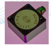
The AMB range of accelerometers are Biaxial MEMS (micro electro mechanical system) DC response voltage output devices for testing at low frequency vibration measurement from DC (0Hz) and above. They are Biaxial (measuring in 2 directions simultaneously) variable capacitance design. The AMB/10.200C has a 4 pin ½-28UNF side entry connector.
