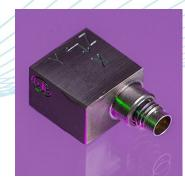
A lightweight general purpose triaxial vibration transducer comprising of three voltage output piezo-electric sensing elements mounted orthogonally within a titanium block with welded construction. The ATI/14/TB is based upon the unique DJB Konic shear® design.
