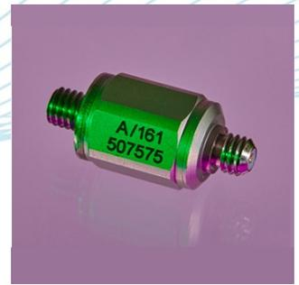
Developed for demanding applications requiring the measurement of high amplitude, short duration transient events such as pyrotechnic shock or high energy impacts, the A/16X range of stainless steel IEPE accelerometers have a range from 10,000g up to 50,000g.
