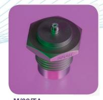
A smaller pressure transducer, doubling acoustic bandwidth, but at expense of 14dB reduction in sensitivity, thus 0.01pC noise equivalent acoustic signal threshold increases to 82dB (2.5mbar) M/02 application areas measurement, blast include air combustion gas acoustic measurement, fluid flow dynamics. Signals may be superimposed upon high static pressure backgrounds. Transducers are calibrated at ambient pressure.
