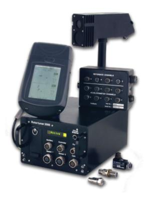
Unique 'windowed' vibration ranges may be configured to create very high resolution FFT's. This facilitates discrimination between closely matched frequency sources for specific aircraft diagnostic requirements. Supplementary techniques include a dedicated vibration absorber-tuning programme.
