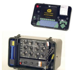
system is EMC compliant with Mil Stan 461E and UK Def. Stan. 59-41 ("above decks" compliant). The RT- 5JS+ also has an extended operating temperature range from -25°C to +55°C.
